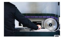
A crossbelt system with counterrotating abrasive blocks is used to make edge rounding on laser, punch, shear or waterjet cut parts.
