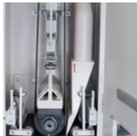
__ FC120 Z has one abrasive belt unit
