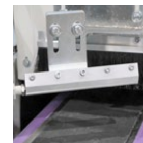
__ air blower: reducing the quantity of splashes outside of the machine
