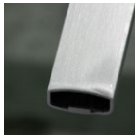
__ FGWH170 8Z finishes all four sides simultaneously
