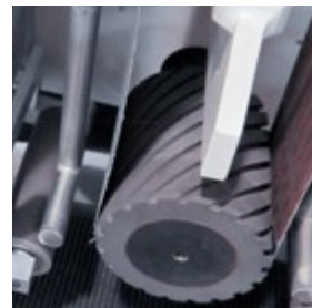
— water cooling reduces the heat on the grinded material
