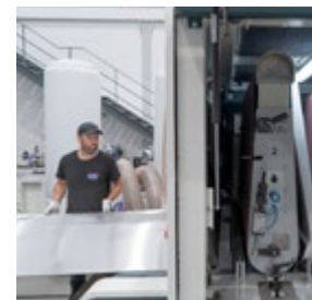
___ double or triple abrasive belt station plus finishing brush (2ZK and 3ZK)
